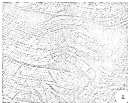
Fig. 8. Fracture of beryllium single crystals at T = 500^\circ\text{K} , \delta_{tot} = 27.3\% , \sigma_b = 124 \text{ kg/mm}^2 . a) Longitudinal bending of (0001) layers with formation of cracks in the basal plane; (x 340). b) Principal elements of fracture: (1\bar{2}14) , (11\bar{2}0) , and (0001) . (x 200).
